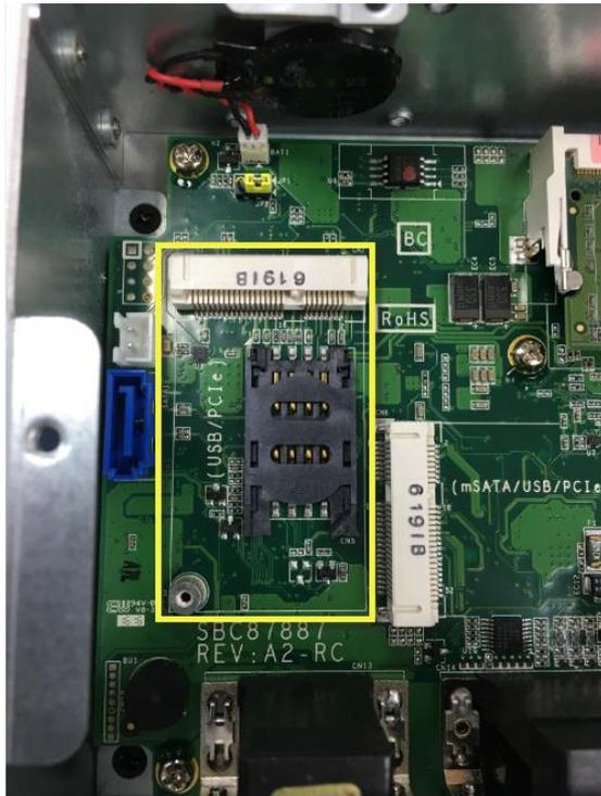
**Step4** Following (Figure 4-1) push the SIM slot back to unlock SIM slot, inserting the SIM card and put it back(Figure 4-2), and lock the SIM slot(Figure 4-3).
