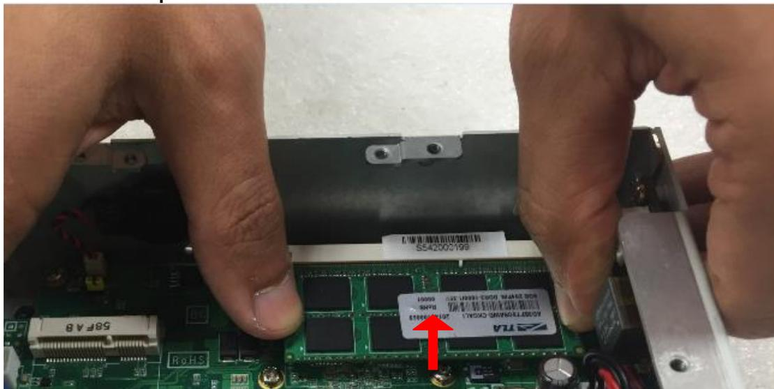
**Step 4** The memory module is locked by two latches on the sides. We strongly recommend using “LDC737” silicone on the two sides of the memory for good ability of vibration.
