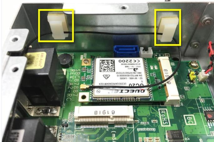
**Step9** Taking out the parts from the 3G kit package and screws tight it.
