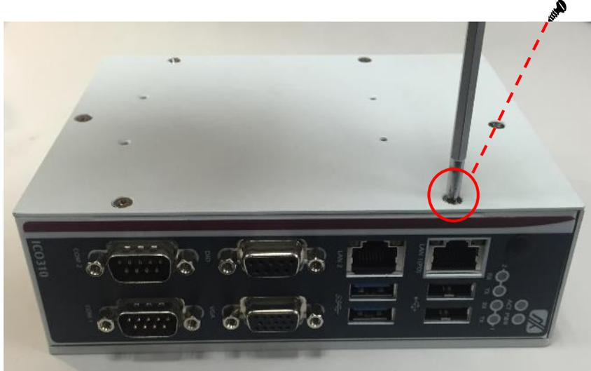
**Step 3** Loosen 4pcs screws of the cover, and put the HDD into the HDD bracket and fix the HDD by 4pcs of screws in the accessory bag.
