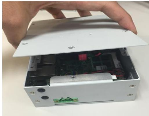
**Step 6** Put the cover back to the system, and fasten screws tight close the chassis.
