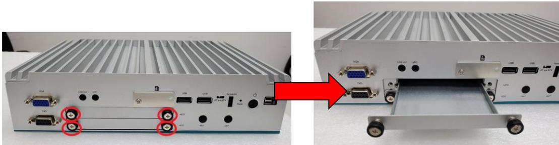
**Step 3** Turn the SATA drive tray upside down to install SSD/HDD and then fasten the four HDD screws to secure the SATA drive tray.
