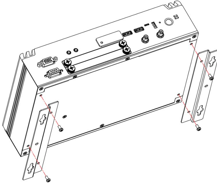
Note : If users install the screws in drywall, use the hollow wall anchors to ensure that the unit does not pull away from the wall due to prolonged strain between the cable and the power connector.
