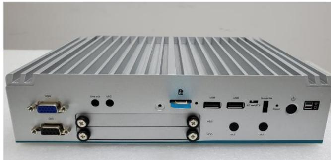
SIM card direction (contact side facing upward)
