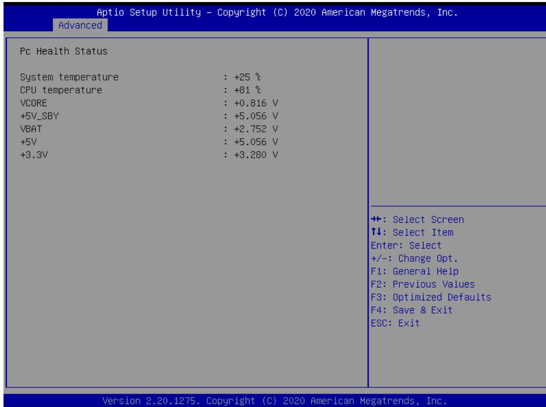
This screen displays the temperature of system and CPU as well as system voltages (VCORE, +5V STBY, VBAT, +5V and +3.3V).
