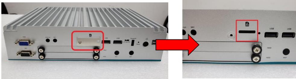
**Step 3** Make sure the SIM card direction is correct and insert the SIM card firmly.
