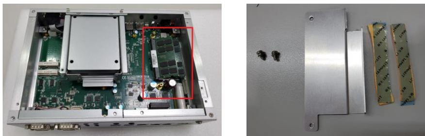
**Step 5 Please place the DRAM thermal pad on the module and screw the bracket.**
