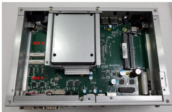
**Step 4** Slot A is used as the wireless mini card slot, insert the WiFi or LTE mini PCIe module into the slot and fasten the screw.
