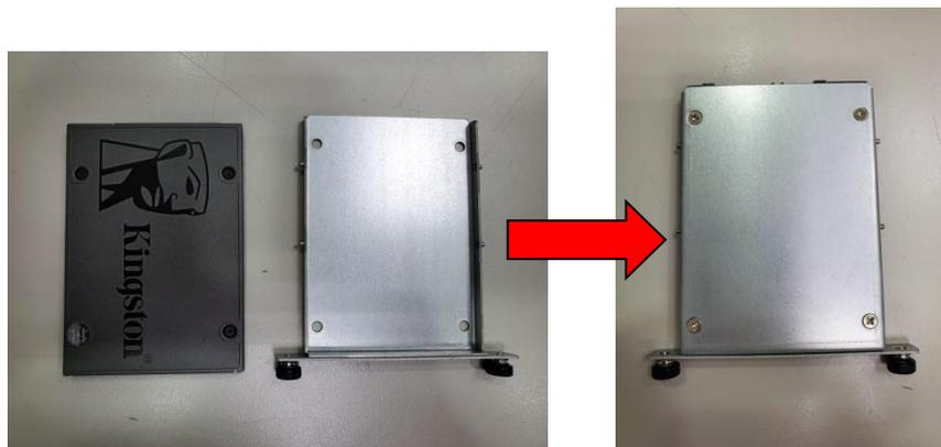
**Step 4** Slide the SATA drive tray back into the system and fasten the screws firmly to complete the installation.
