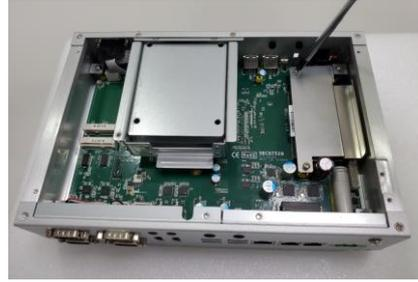
**Step 6 Put the bottom cover back and fasten two screws back onto the system.**
