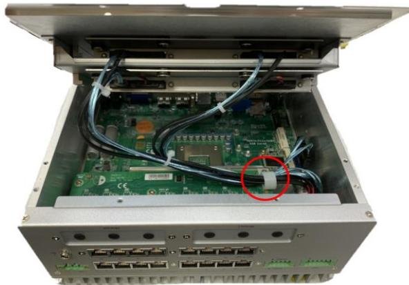
**Step 5 Insert the PCIe card and fasten the screws as shown.**
