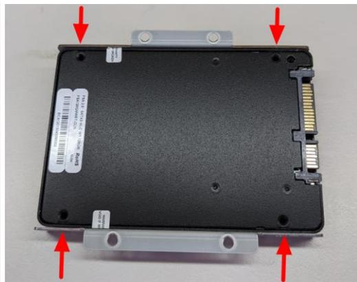
**Step 4** Install the HDD tray back to the system cover. Connect the SATA cable between HDD and MB.
