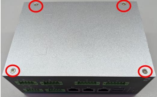
**Step 3** Loosen 4pcs screws of the HDD tray, and fix the HDD into tray with screws.
