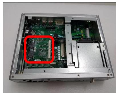
**Step 4 Assemble I/O cable to fix the I/O bracket then fasten dual screws of the Flexible I/O Window.**
