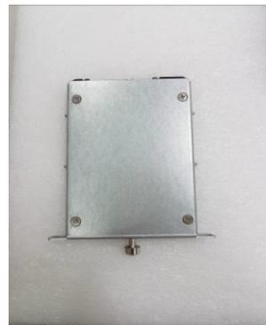
**Step 4** Slide the SATA drive tray back into the system and fasten the screws firmly to complete the installation.
