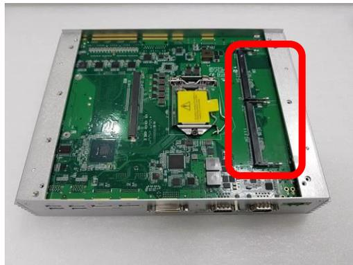
**Step 4** Locate the memory module, insert a gold colored contact into the socket and push the module down until it is locked in place by the two end latches.
