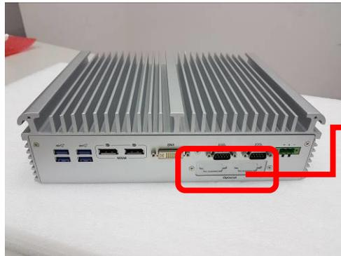
Flexible IO Window for mPCIe IO kits
