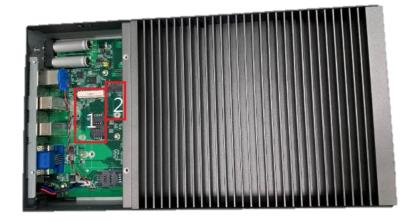
**Step 5** Remove the antenna plug from the front side, and then install the antenna on the antenna connector. The installation is complete.
