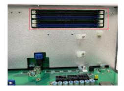
The supports an optional bracket to avoid memory module bounced off from sockets. Please refer to the following instructions and illustrations for installation.
