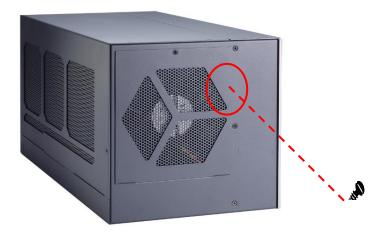
**Step 4** Take the fan module and its screws from the accessory box.
