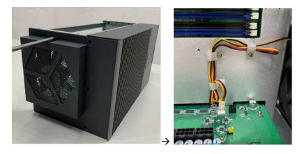
**Step 7** Close the side cover back to the chassis and fasten all screws. The installation is complete.
